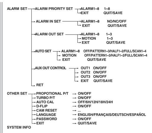
The diagram shown above illustrates the overall structure of the Setup Menu. In this section, a description of the Setup menu features will enable users of the SCC-C6407(P) to tailor it to their personal needs.
